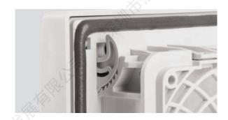
The Filter Fan Plus is placed in the enclosure cut-out from the outside of the enclosure and mounted tool-free. By pressing the built-in ratchet braces the filter fan is pulled into the cabinet wall. The ratchet braces snap into place, giving the installer audible feedback that the filter fan is now installed securely. The ratchet mount is suitable for a wall thickness from 1 to 4 mm.
